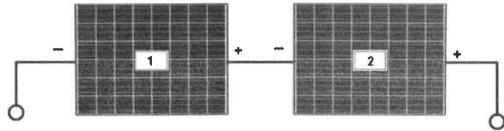
Fig. 1.1: Two dissimilar PV modules connected in series.
