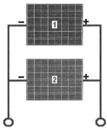
Fig. 1.2: Two dissimilar PV modules connected in parallel.
