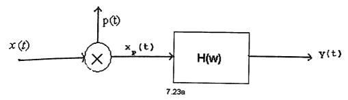
The sampling signal p(t), the Fourier Transform of the input signal x(t) and the frequency response of the filter  $H(\omega)$  are shown below:
