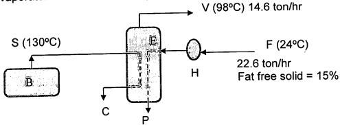
S = steam, P = product, F= feed, H = heater, B = boiler, E = evaporator, C = condensate, V = vapour
