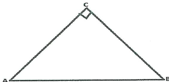
The distance AB must be 10m and the angle ACB must be 90 degrees. The lengths of the other two sides, AC and BC must total 13m.
